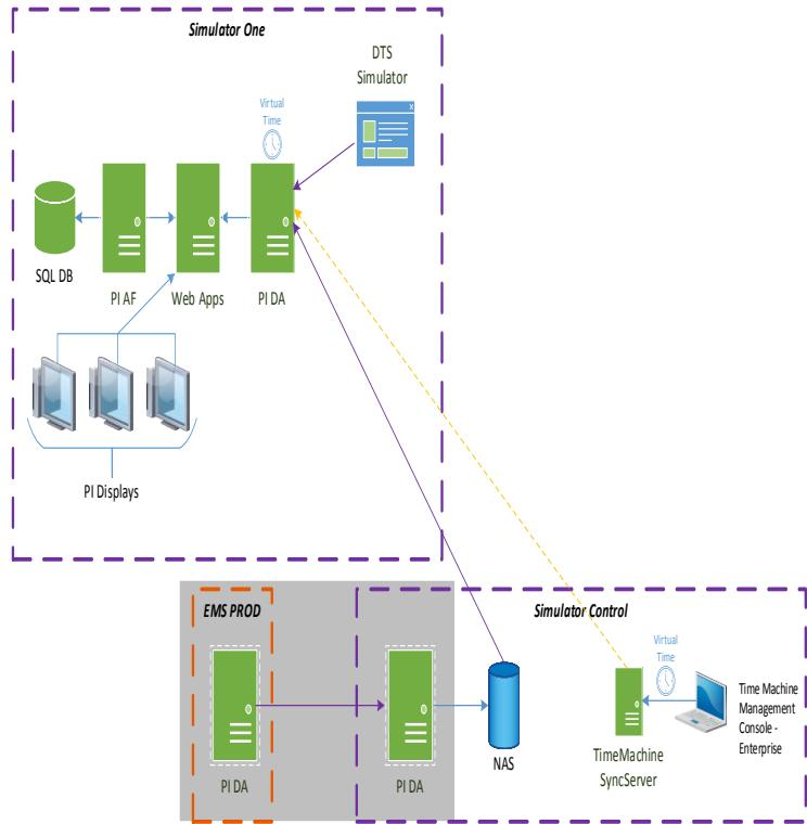
**POC Diagram:** Time Machine Sync Server synchronizes virtual time across distributed servers without altering system clocks.
