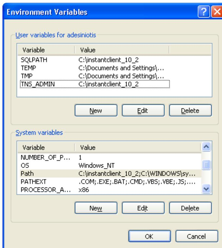
8. Create 2 new “User Variables” called **SQLPATH** and **TNS\_ADMIN** with the installed client folder **C:\instantclient\_10\_2** as the Variable Value
